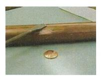
Your Service Line is Copper if: Scratch Test: Area is copper in color like a penny. Magnet Test: Does not stick.
